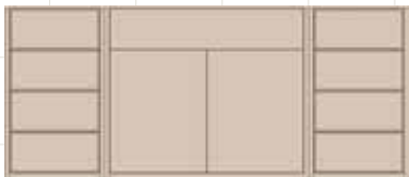
TILLI VANITY (VA04) W 72.75 D 22 H 30.75 (+base) One Non-Functional Top Drawer in Center, Eight Drawers - Standard with Outside Bead Face Only, Two Doors Fits Standard 73" Vanity Top, Single Basin or VA04T Note: Must select two hardware placements
